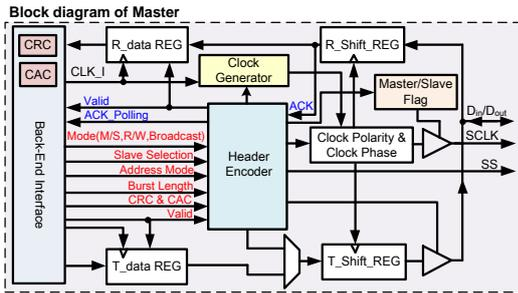
Fig. 4. Block diagram of master module.
