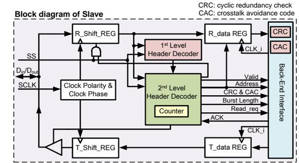
Fig. 4. Block diagram of slave module.
