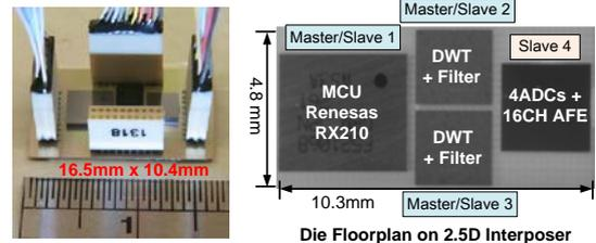
Fig. 5. 2.5D heterogeneously integrated bio-sensing microsystem.
