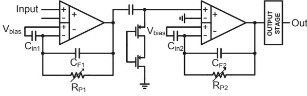
Fig. 2. Schematic of 1-Channel AFE.
