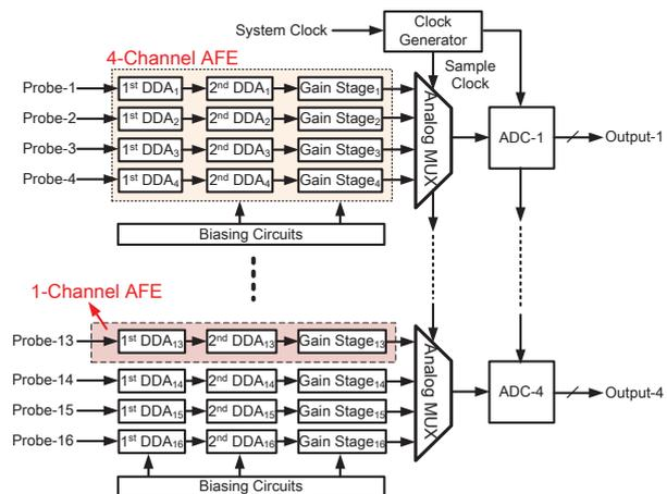
Fig. 1. 16-channel AFE with 4 ADCs for neural signal acquisition
