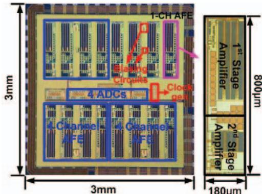
Fig. 8. Chip microphotograph of 16-channel AFE with 4 ADCs.
