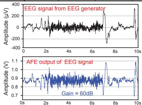
Fig. 10. (a) The original EEG signal (b) The output signal from ADC.
