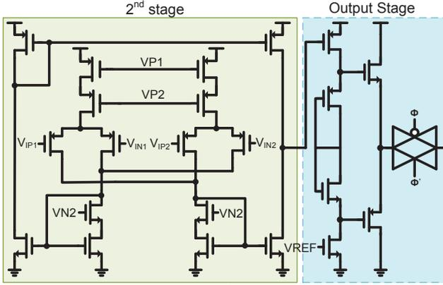
Fig. 5. Schematics of 2<sup>nd</sup> stage & output stage
