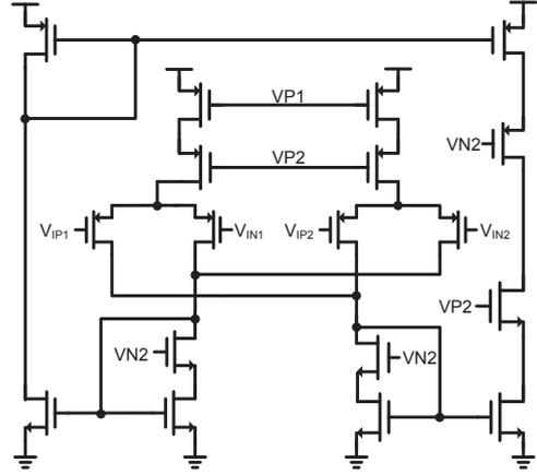
Fig. 4. Schematic of 1<sup>st</sup> DDA stage.
