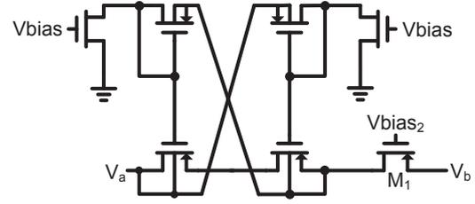
Fig. 6. Schematic of pseudo resistor with M1.
