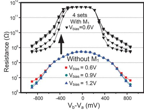
Fig. 7. Resistance of pseudo resistors with/without M1.
