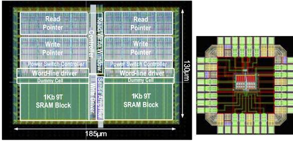
Fig. 10. Floorplanning and the layout view of the proposed FIFO memory.
