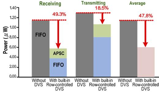
Fig. 11. Comparisons of the power consumption with/without the built-in row-controlled DVStechnique.
