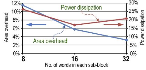
Fig. 8. The area overhead and power dissipation with different sub-block size.
