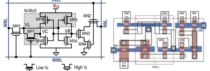
Fig. 9. Schematic and layout of the 9T SRAM bit-cell.
