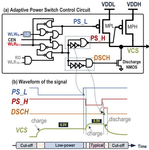
Fig. 6. Adaptive power switch unit and the corresponding waveform.
