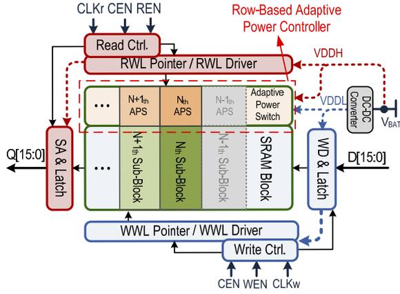
Fig. 2. block diagram of the built-in row-controlled DVS FIFO memory.
