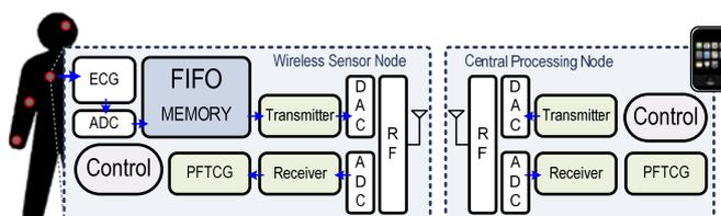
Fig. 1. Block diagram of WSN and CPN for WBAN.
