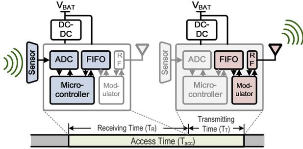
Fig. 3. The receiving time and transmitting time of FIFO in WBAN systems.
