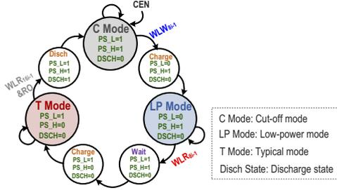
Fig. 7. FSM of the row-based adaptive power control.
