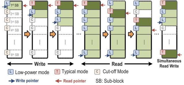
Fig. 5. Operation examples of the built-in row-controlled DVS FIFO.
