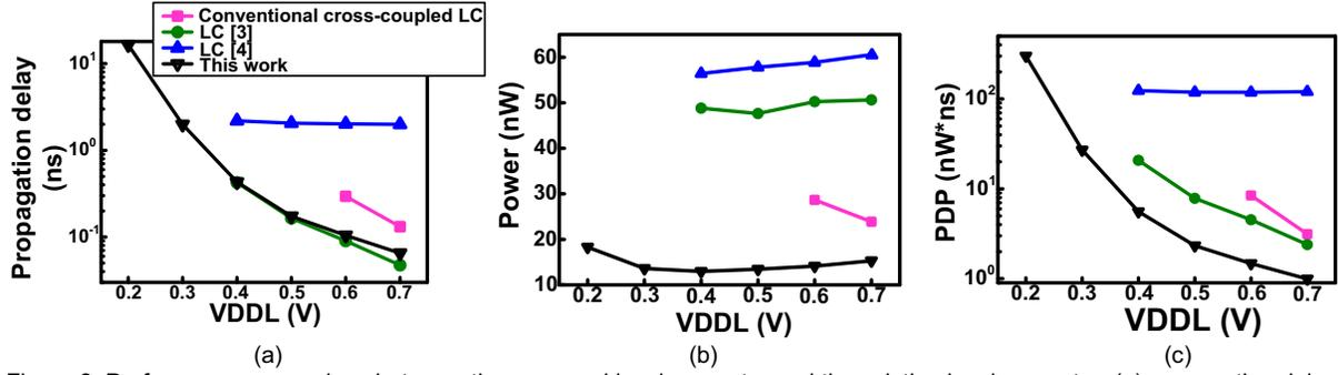
Figure 8: Performance comparison between the proposed level converter and the existing level converter: (a) propagation delay comparison (b) power comparison (c) PDP comparison
