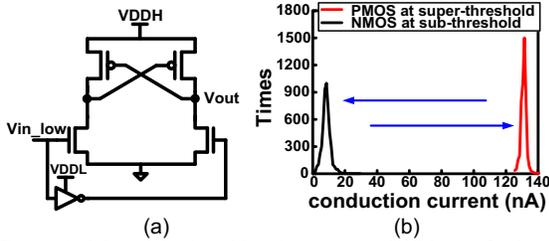
Figure 1: (a) conventional level converter (b) Monte Carlo simulation of conduction current
