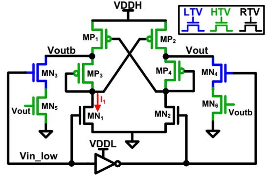
Figure 2: Schematic view of the proposed level converter
