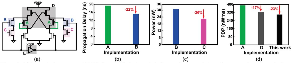
Figure 4: (a) A: two diode-connected PMOS. B: multi- $V_{th}$  devices. C: leakage reduction technique. D: reverse short channel effect. E: inner inverter sizing. (b) By implementation B, delay reduction up to 22% (c) By implement C, power reduction up to 26% (d) By implement D, PDP reduction up to 17%. Finally, combining all implementation, overall PDP reduction up to 23%
