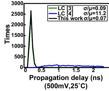
Figure 9: Monte Carlo simulation for propagation delay when supply voltage is 500mV
