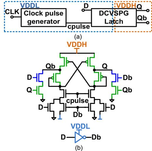
Figure 6: (a) The proposed dual edge-triggered explicit-pulsed level-converting flip flop. (b) A modified DCVSPG latch
