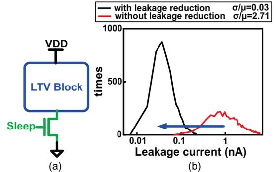
Figure 5: (a) leakage reduction technique [11] (b) Monte Carlo simulation of leakage current with/without leakage reduction technique
