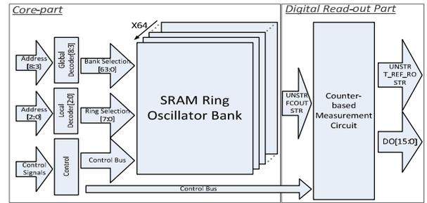
Fig. 10. Block diagram of the whole system.
