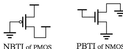
Fig. 1. NBTI stress of PMOS and PBTI stress of NMOS.
