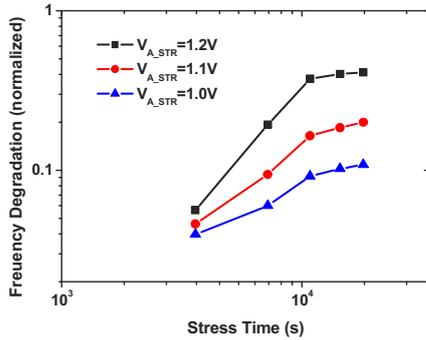
Fig. 11. Measured ESRO frequency degradation versus stress time for different NBTI stress voltage.
