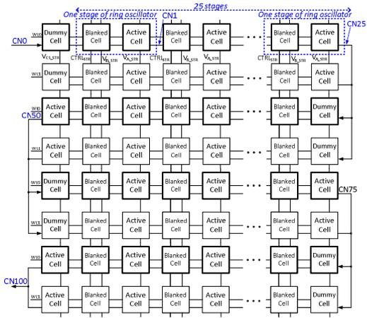
Fig. 6. 100-stage ESRO chain composed of modified SRAM cells.
