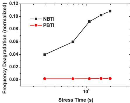
Fig. 12. Measured ESRO frequency degradation under NBTI-only and PBTI-only stress in SiO<sub>2</sub>/poly-gate technology.
