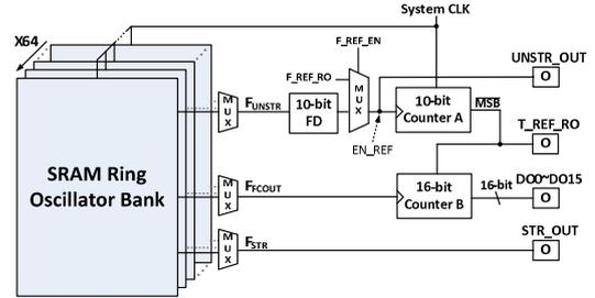
Fig. 9. The counter-based digital read-out measurement scheme.
