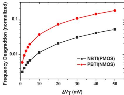
Fig. 7. Simulated frequency degradation vs. threshold voltage drift.
