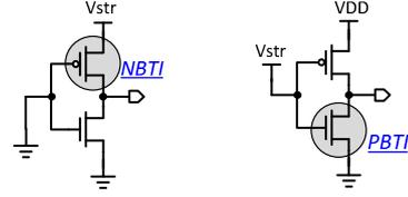
Fig. 3. One stage inverter under stress of NBTI and PBTI.
