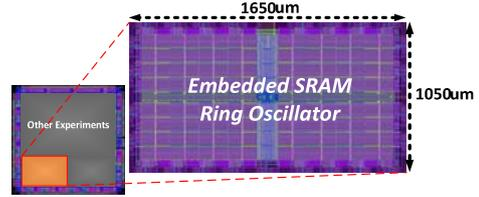
Fig. 13. Die photo (left) and layout view (right) of the test chip.
