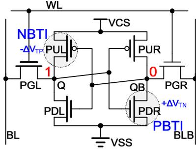
Fig. 2. A 6T cell suffers asymmetrical degradation from NBTI and PBTI.
