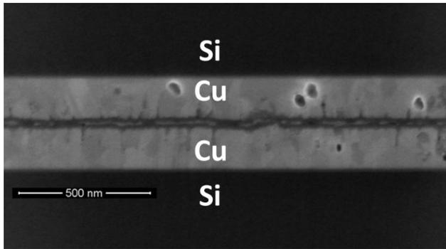
**Figure 11.** SEM image of Cu/Cu bonded interconnect with Ti passivation.
