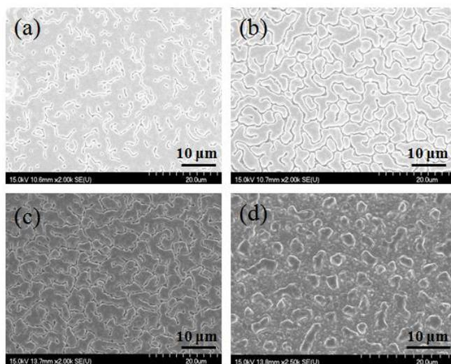
**Figure 1.** The surface morphology of In coating on (a) SiO<sub>2</sub>, (b) Ti, (c) Ni/Ti, and (d) Cu/Ti.
