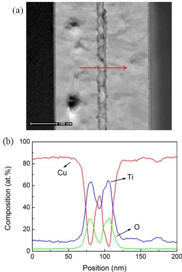
**Figure 12.** (a) TEM image of the Cu/Cu bonded interconnect with Ti passivation and the EDX scanning direction; (b) composition profile obtained by EDX line-scan.
