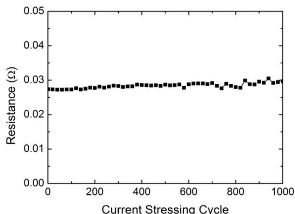
**Figure 8.** The measured resistance of Cu/In bonded interconnect under current cycling test.
