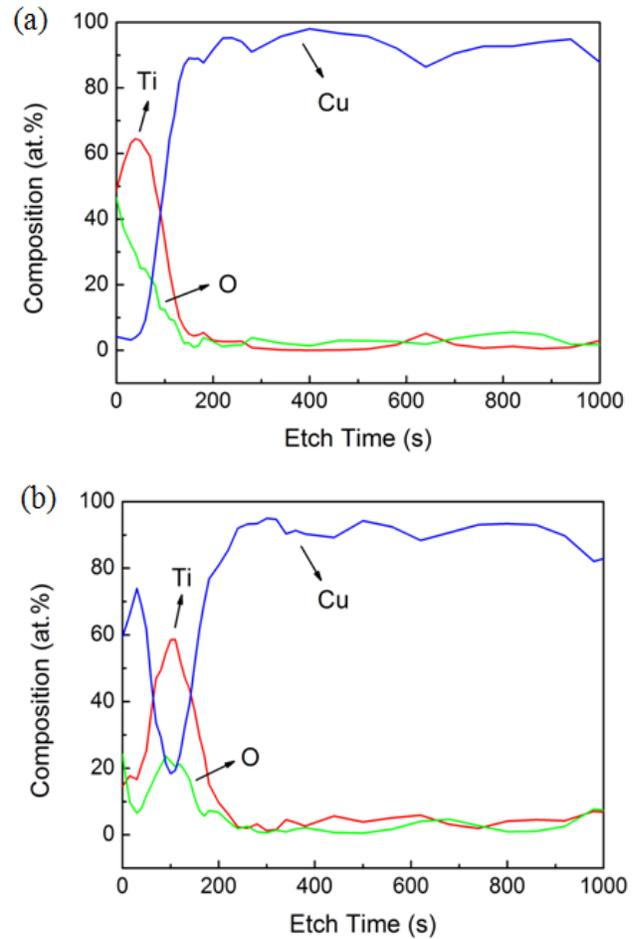
**Figure 13.** Auger depth profile of bonded structure (a) before annealing, and (b) after annealing at 400°C for 60 min.
