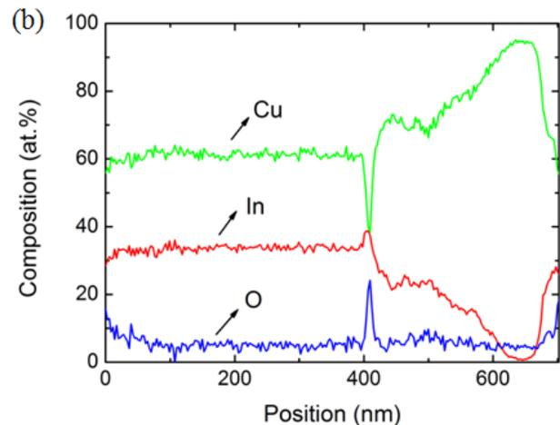
Figure 6. (a) TEM image of the Cu/In bonded interconnect and the EDX scanning direction; (b) composition profile obtained by EDX line-scan.
