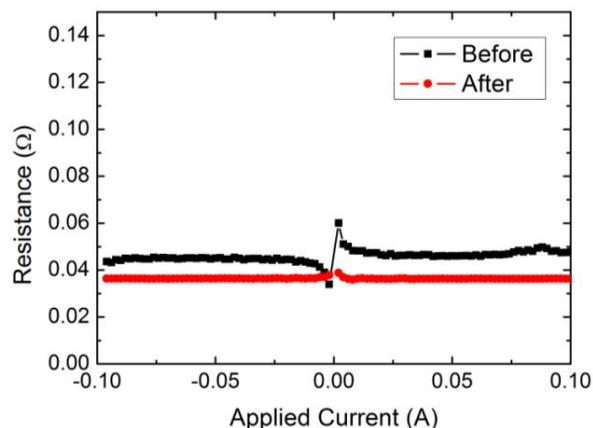
**Figure 10.** The measured resistance of Cu/In bonded interconnect under humidity test.
