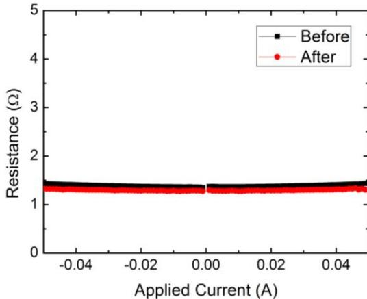
**Figure 15.** The measured resistance of Cu/Ti-Ti/Cu bonded interconnect under temperature cycling test.
