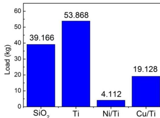
**Figure 3.** The shear test results of In/In bonding with different adhesive materials.
