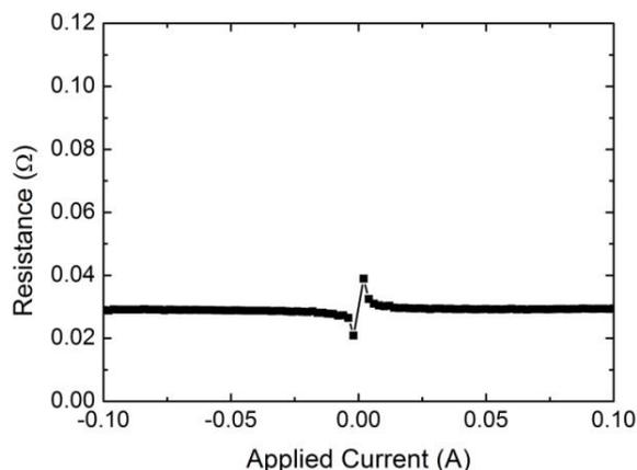
**Figure 7.** The measured resistance of Cu/In bonded interconnect.
