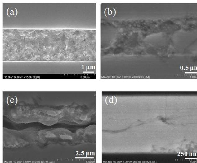
**Figure 2.** In/In bonding with different adhesive materials: (a) SiO<sub>2</sub>, (b) Ti, (c) Ni/Ti, and (d) Cu/Ti.
