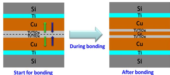
**Figure 14.** Schematic diagram of the Cu/Ti-Cu/Ti bonding procedure.
