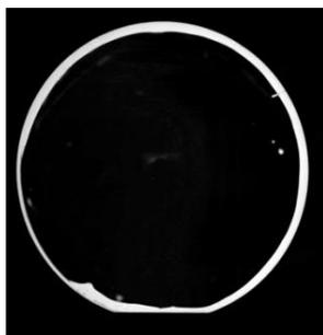
Figure 5. SAT image of 4" Cu/In wafer bonding result.
