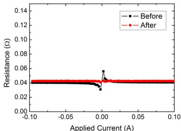
**Figure 9.** The measured resistance of Cu/In bonded interconnect under temperature cycling test.
