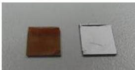
Fig. 2 Cu-Sn bond failure samples from group 1 with HCl cleaning bonded.
