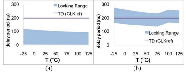
Figure 20. PVT compensation for locking range of clock generator at 0.5V FF corner (a) before compensation, (b) after compensation.
