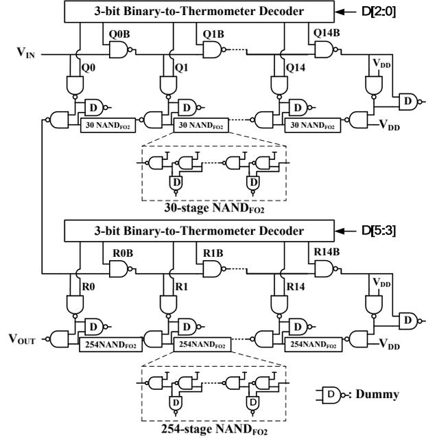
Figure 8. PVT compensation delay line.
