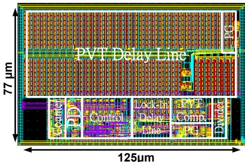
Figure 21. Layout view of the proposed clock generator.
