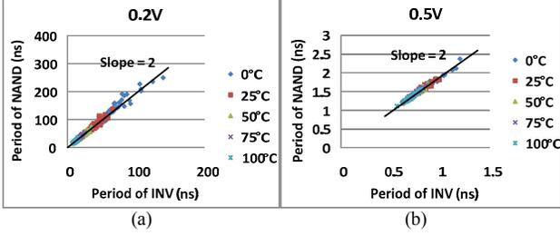
Figure 10. Monte Carlo simulations for periods of ring oscillators (composed of FO1-INV and FO2-NAND) (a) at 0.2V, (b) at 0.5V.
