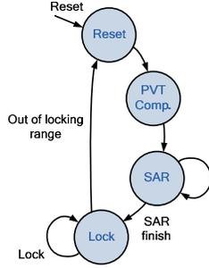
Figure 3. Proposed finite state machine (FSM).
