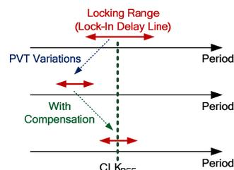
Figure 1. Concept diagram of PVT compensation.
