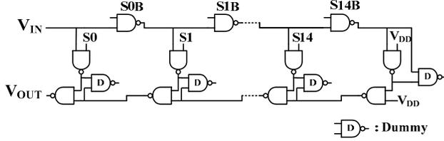
Figure 6. Topology of delay line (lattice delay line [4]) used in the proposed clock generator.
