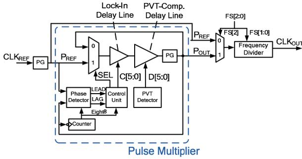
Figure 2. Proposed clock generator for near-/sub-threshold DVFS system.
