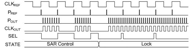
Figure 5. Timing diagram of the proposed FSM operating from SAR to Lock state.
