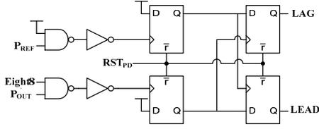
Figure 14. Phase detector.
