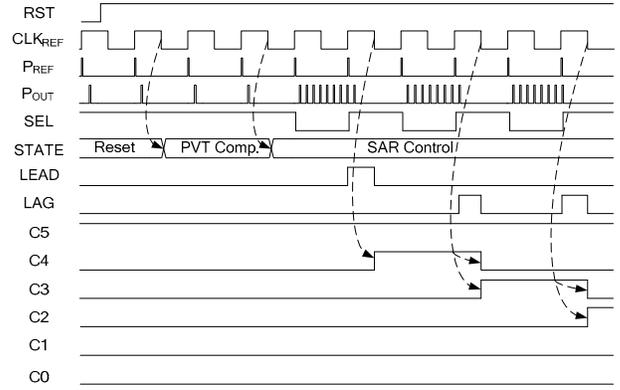
Figure 4. Timing diagram of the proposed FSM operating from Reset to SAR state.
