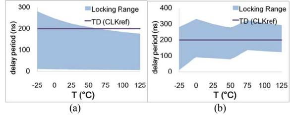
Figure 19. PVT compensation for locking range of clock generator at 0.5V TT corner (a) before compensation, (b) after compensation.
