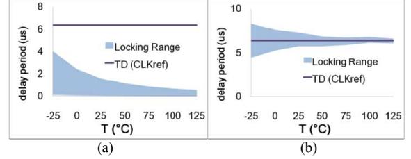
Figure 18. PVT compensation for locking range of clock generator at 0.2V FF corner (a) before compensation, (b) after compensation.
