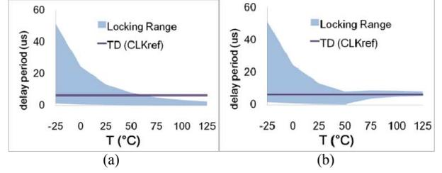
Figure 17. PVT compensation for locking range of clock generator at 0.2V TT corner (a) before compensation, (b) after compensation.
