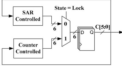
Figure 11. Lock-in delay line controller.
