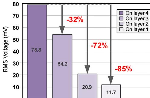
Fig. 7. Noise comparison with different analog layer.
