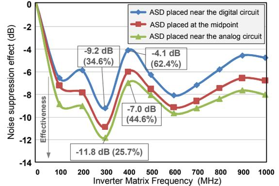
Fig.5. Noise suppression effect on mixed-signal layer.
