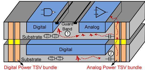
Fig. 1. Two propagation paths of substrate noises in 3D ICs.
