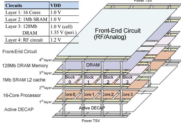
Fig. 9. Heterogeneous TSV 3D integration with multi-core, SRAM, DRAM, front-end circuits stacking.
