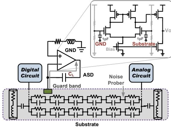
Fig.2. Schematic of active substrate decoupler (ASD).
