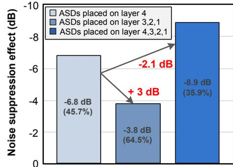
Fig.4. Noise suppression effect of ASD planning for mixed-signal circuit in 3D structure.
