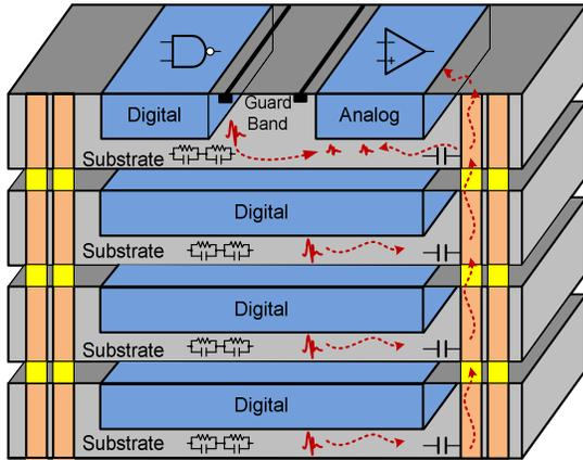
Fig.3. Block diagram of mixed-signal circuit in TSV 3-D integration.
