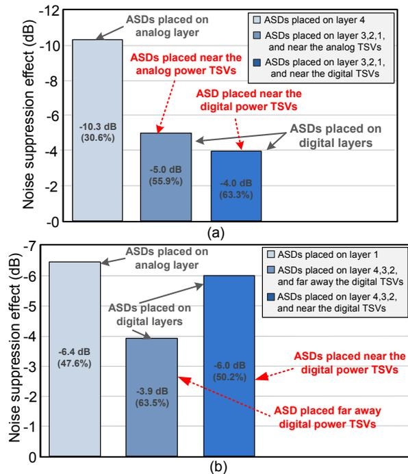
Fig. 8. Noise suppression effect (a) Analog circuit on the top layer. (b) Analog circuit on the bottom layer.
