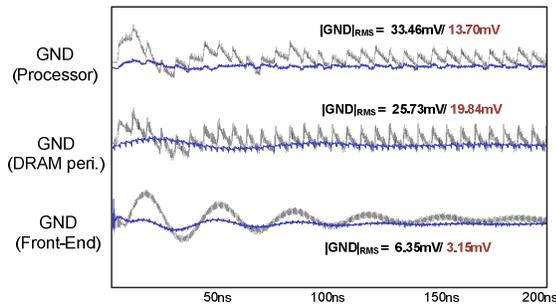
Fig. 10. Waveforms of ground noises with(blue)/without(gray) ASDs.
