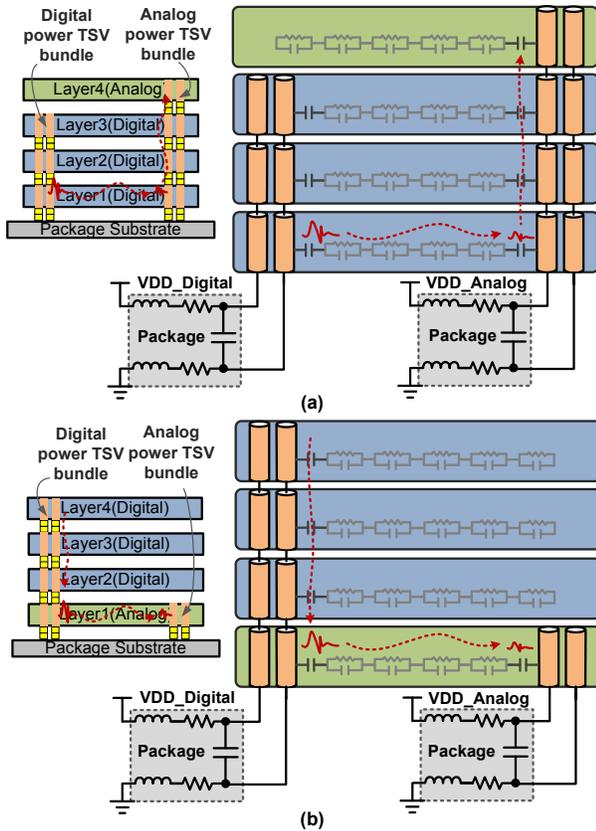
Fig. 6. TSV in 3-D integration. (a) Analog circuit on the top layer. (b) Analog circuit on the bottom layer.
