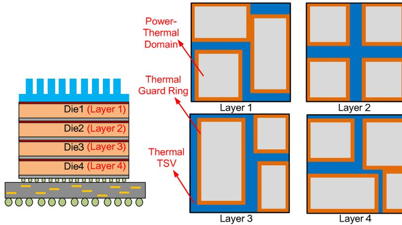
Fig. 8. Power-thermal domain setup in a 4-layer TSV 3D-IC with back-to-face bonding technique.
