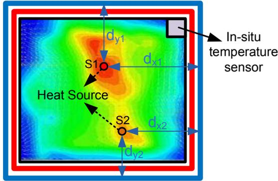
Fig. 5. Temperature detection with analytical model.
