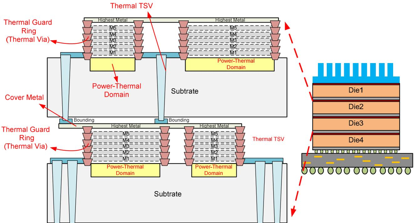
Fig. 2. Thermal control mechanism for TSV 3D-ICs is proposed using thermal guard rings, a cover metal and thermal TSVs.
