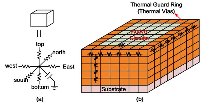
Fig. 7. (a) Equivalence electrical RC of a cube (b) Thermal dissipation model with the thermal guard ring
