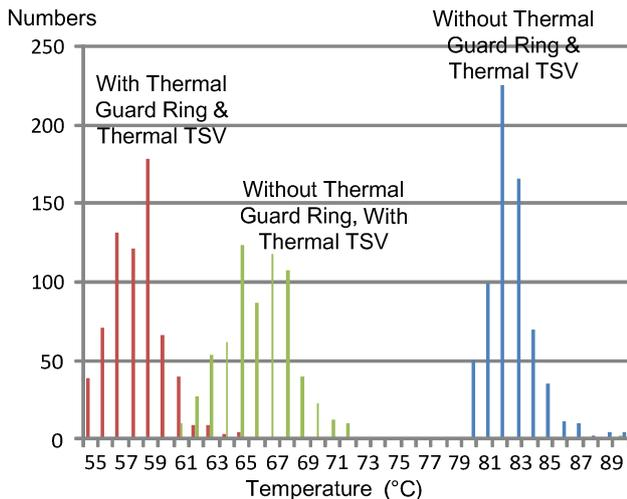
Fig. 10. Temperature scatter graph of layer-3 in the three TSV 3D-IC structures.
