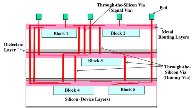
Fig. 1. Cross-Section of a TSV 3D-IC with thermal TSVs. [4]
