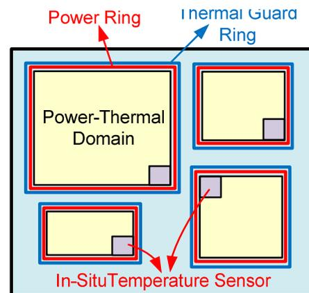
Fig. 3. Power-thermal domains with in-situ temperature sensors.
